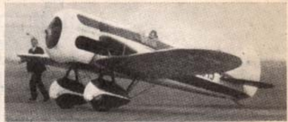
Travel Air „Mystery Ship“. V_{max}=378 km/t, N/F=35 hv/m 2 .
